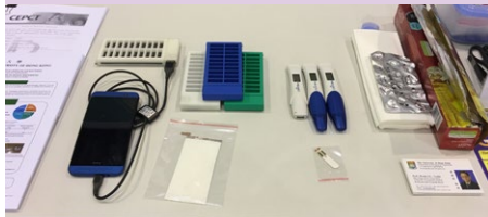
Innovative paper-based aluminum-air batteries developed by the research team of Professor D.Y.C. LEUNG.
